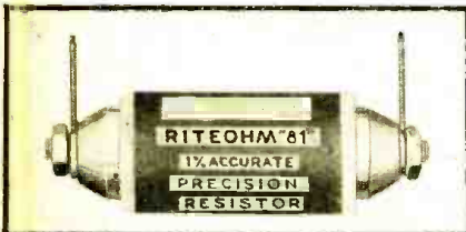
New line of "pie-wound" precision resistors. (1568)
